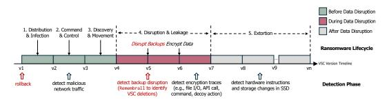
Fig. 5. Ransomware lifecycle stages and corresponding mitigation efforts. Our work targets an unexplored phase - detecting backup disruption - where current approaches fall short, distinct from previous research on network traffic, encryption traces, SSD logs, etc.
