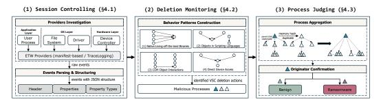
Fig. 1. Overall workflow of REMEMBRALL. It contains three modules: Session Controlling, Deletion Monitoring, and Process Judging. If ransomware is detected, all corresponding processes will be killed, and the system backup disruption attack (i.e., VSCs deletion) will be terminated.
